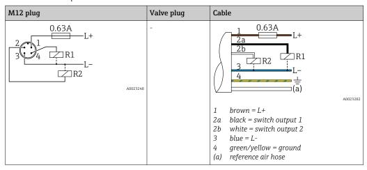
*IO-Link: 2 x PNP switch output R1 and R2*
