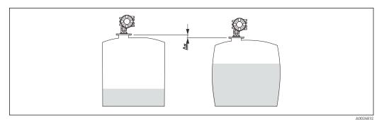
$\blacksquare$  19 Movement  $\Delta x$  of the tank reference height due to the bulging of the tank shell caused by hydrostatic pressure
