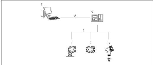
**■** 17 Remote operation of Tank Gauging devices
