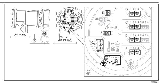
$del{1}$  Terminal compartment (typical example) and ground terminals
