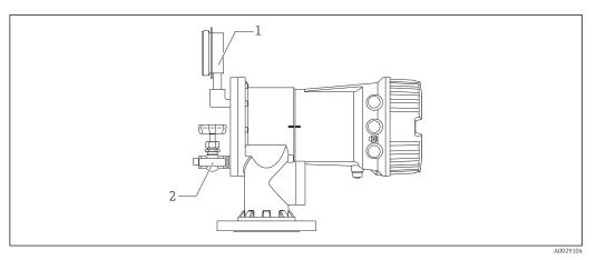
23 Mounting position of relief valve and pressure gauge
