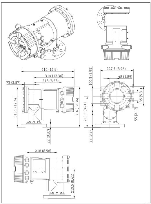
The thickness of the flange (22 mm (0.87 in)) shows the specification of the 10K 150A RF aluminium flange JIS B2220.
