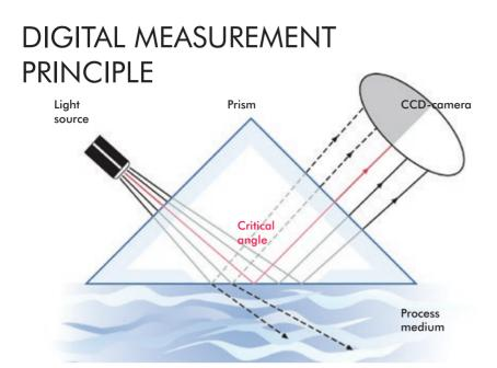
The light source sends light against the interface between the prism and the process solution, where the rays meet the surface at different angles.
