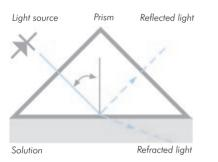
Depending on the angle, some rays are totally reflected. Some rays are only partially reflected, and most of the light is refracted into the process solution.
