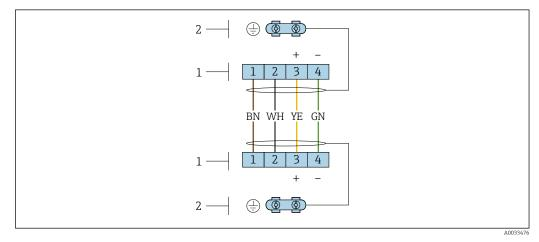
🖲 3 Terminals for connection compartment in the transmitter wall holder and the sensor connection housing
