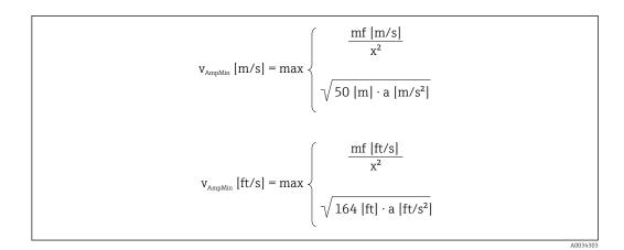
$v_{\textit{AmpMin}} \quad \textit{Minimum measurable flow velocity based on signal amplitude}$
