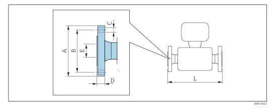
Length tolerance for dimension L in inch: DN  $\leq$  4": +0.06 to -0.08 in i  $DN \ge 6$ ": ±0.14 in
