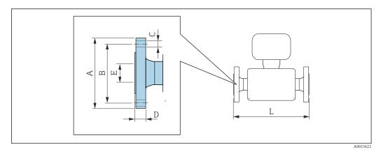
Length tolerance for dimension L in mm: DN ≤ 100: +1.5 to -2.0 mm DN ≥ 150: ±3.5 mm
