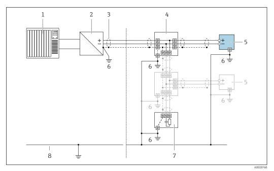
🛃 9 Connection example for FOUNDATION Fieldbus
