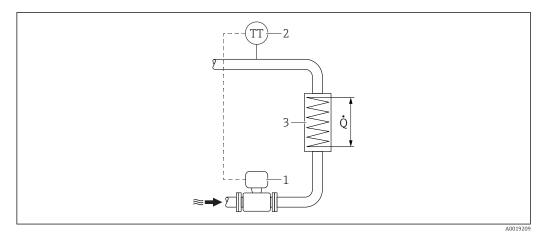
$\blacksquare$  18 Layout for delta heat measurement of saturated steam and water
