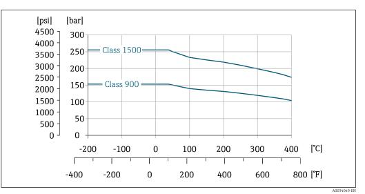
🗷 20 Flange connection material: stainless steel, multiple certifications, 1.4404/F316/F316L
