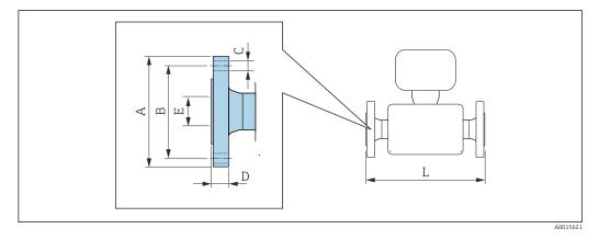
Length tolerance for dimension L in inch:  $DN \le 4^{"}$ : +0.06 to -0.08 in  $DN \ge 6^{"}$ : ±0.14 in
