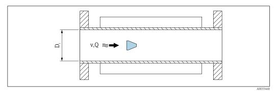
$D_i$  Internal diameter of measuring tube (corresponds to dimension  $K \rightarrow \square 52$ )
