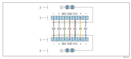
*E* 4 Terminals for connection compartment in the transmitter wall holder and the sensor connection housing
