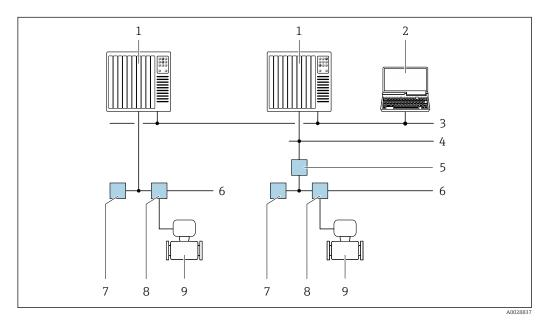
29 Options for remote operation via FOUNDATION Fieldbus network
