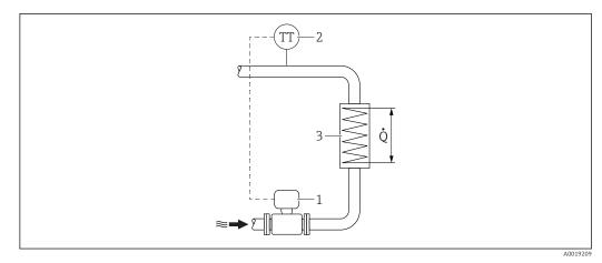
$\blacksquare$  18 Layout for delta heat measurement of saturated steam and water
