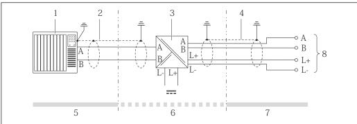
■ 3 Connection example for Modbus RS485 intrinsically safe
