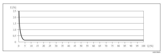
Error: Maximum measured error as % o.r. (example) Ε Q
