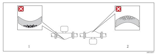
Orientation of sensor with curved measuring tube
