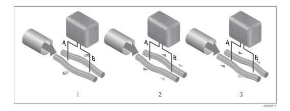
The phase difference (A-B) increases with increasing mass flow. Electrodynamic sensors register the tube oscillations at the inlet and outlet. System balance is ensured by the antiphase oscillation of the two measuring tubes. The measuring principle operates independently of temperature, pressure, viscosity, conductivity and flow profile.
