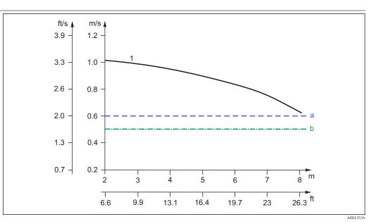
■ 4 Intake speed in m/s with suction height in m
