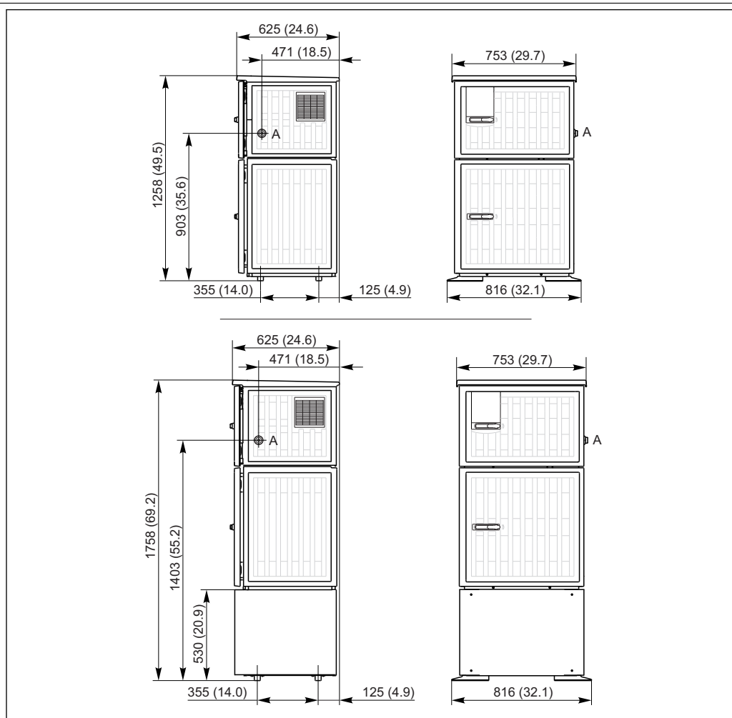
26 Dimensions of Liquistation CSF48 plastic version, without/with stand, dimensions in mm (in)
